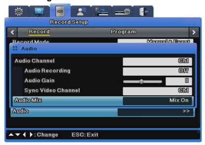
This menu is used to select audio for live video feeds. If All is set, all inputted audio is mixed for output regardless of channel selection. If specific audio is selected, only the specified channel is outputted regardless of the channel selection.
